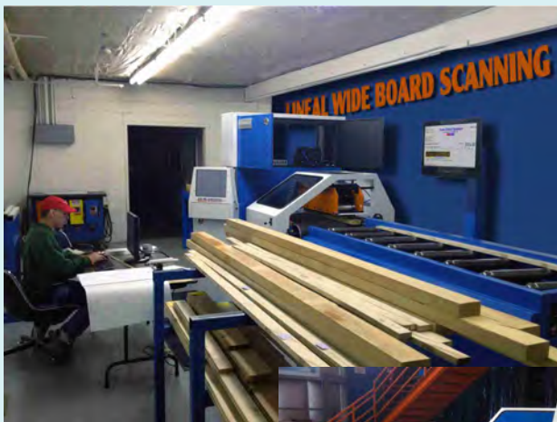
The “Lineal” wide board scanner, and the feed conveyer.
